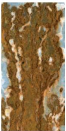
Hot dip galvanized 20µm after 6 weeks
