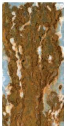
Hot dip galvanized 20µm after 6 weeks
